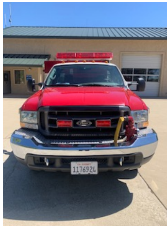
Attack 61 Make: Pierce Model: Type VI Year: 2003 Miles: 17,702 Pump: 150 GPM
