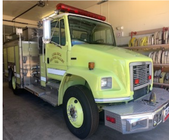
Fire Engine 63 Make: Freightliner Model: Type II Year: 1998 Miles: 49,223 Pump: 1,000 GPM
