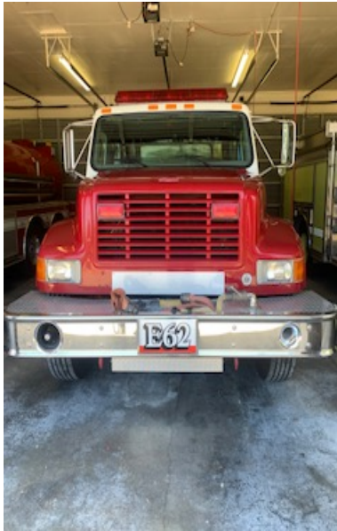
Fire Engine 62 Make: Pierce Model: Type III Year: 2000 Miles: 55,643 Pump: 1,000 GPM
